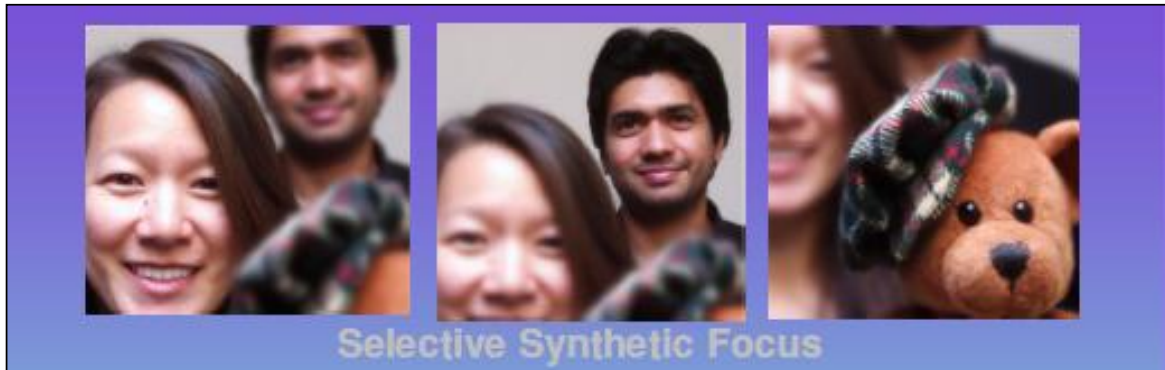
Figure 4. Pelican Imaging’s dynamic focusing. On the left, notice the girl is in focus, in the center the guy in the back is in focus and on the right the teddy bear is in focus – all images dynamically made from Pelican’s 16-array images.
